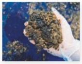
Pour bestabsorb® onto the floating oil and remove - the water is practically as clean as before. The crumbly mass doesn't stick, doesn't grease and can be disposed of without any problem.
